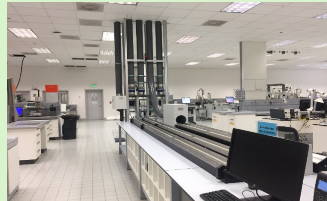
Horizontal conveyors for receive & send: - sort into Priority, Normal & Return lanes
